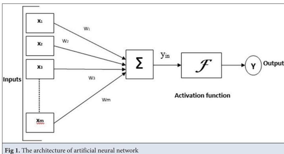
Fig 1. The architecture of artificial neural network
