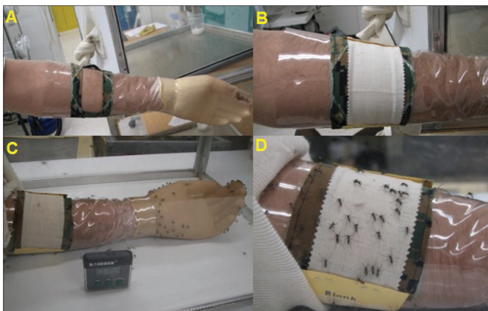
Fig 1. Cloth patch assay (Photo by Greg Allen, Natasha M. Agramonte, Ulrich R. Bernier, USDA, ARS, CMAVE). A- The plastic sleeve that has a 32 cm 2 window previously cut, B- The arm with the sleeve/cloth assembly. The sample to be tested is applied to the cloth, C- The arm with the sleeve/cloth assembly is inserted into a cage containing approximately 500 female Ae. aegypti mosquitoes, and waited for 1 min, D- Failure of repellent treatment is determined by 1% bites (i.e. the volunteer receives 5 bites, for 500 mosquitoes) through the cloth on the sleeve window within 1 min
