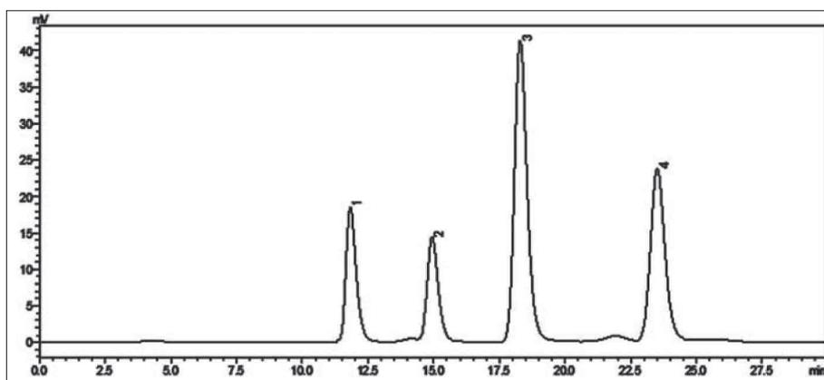
**Fig 1.** HPLC-FLD chromatogram of total aflatoxin standards at a concentration of 2.5 ng/ml. 1- AFG<sub>2</sub>, 2- AFG<sub>1</sub>, 3- AFB<sub>2</sub>, 4- AFB<sub>1</sub>
