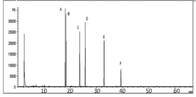
**Fig 3.** Chromatogram of spiked sample (50 ng/g) on a HP-5 capillary column: A= $\alpha$ -HCH, B=HCB, C=HC, D=ALD, E=4,4-DDE, F=4,4-DDT
