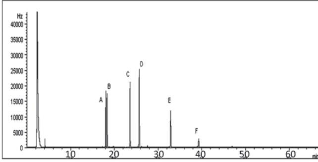
**Fig 2.** Chromatogram of OC pesticide mix standard (25 ng/mL) on HP-5 capillary column: A=  $\alpha$ -HCH, B=HCB, C=HC, D=ALD, E=4,4-DDE, F=4,4-DDT
