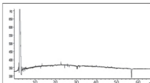
**Fig 1.** Chromatogram of blank sample on HP-5 capillary column
