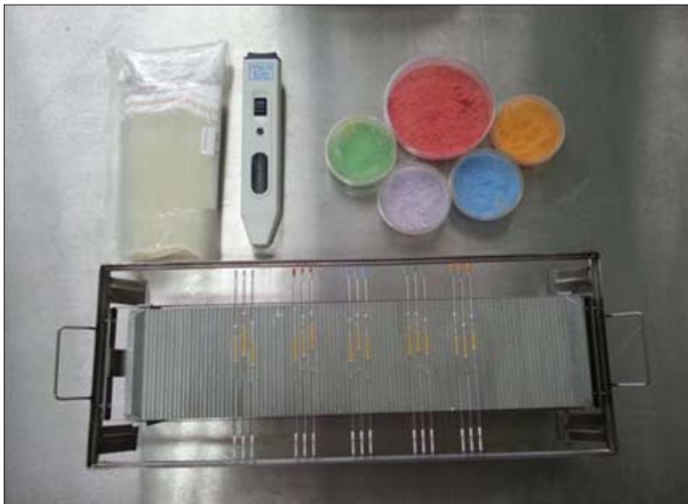
Fig 1. Straws filled and sealed semen with different colors of the polyvinylalcohol (PVA) powder for identification on freezing rack
