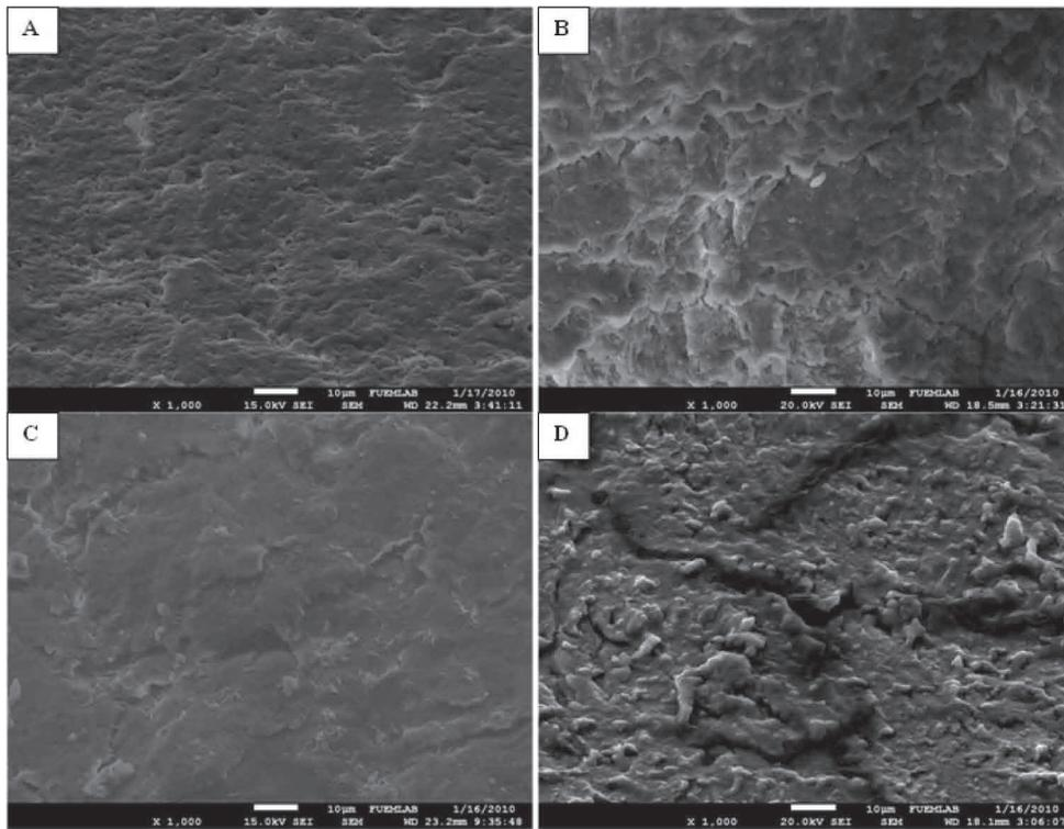
**Fig 4.** SEM views of drilled bone surfaces: A- For drill parameters D=4.5 mm, F=140 N, n=230 rpm, ( $T_{max}=38^{\circ}\text{C}$ ), B- For drill parameters D=4.5 mm, F=140 N, n=1.220 rpm, in dry condition, ( $T_{max}=87^{\circ}\text{C}$ ), C- SEM view for drill parameters of D=4.5 mm, F=40 N, n=570 rpm of the bone sample having density of  $1.739\text{ g/cm}^2$  ( $47.7^{\circ}$ ), D-  $2.430\text{ g/cm}^2$  ( $T_{max}=54^{\circ}\text{C}$ )
