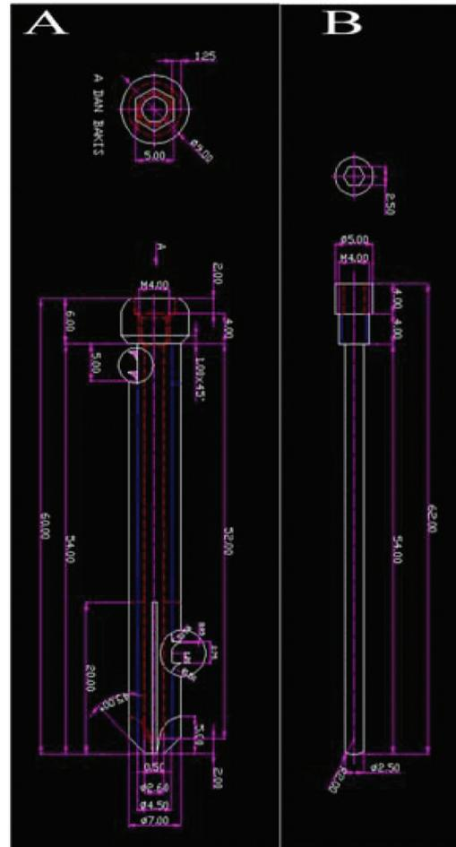
Fig 1. The AutoCAD design of the main component and the second component that allows expansion of the screw
