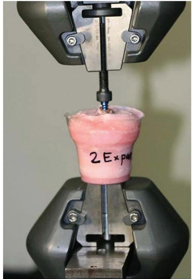
**Fig 4.** Fixing of the screw with methacrylate after insertion into the bone and the connection to the pulling device
