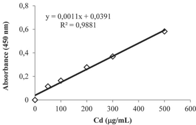
Fig 1. Calibration curve of cadmium adsorption
