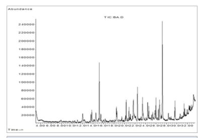
Fig 1. Gas chromatography-mass spectrometry analysis in the essential oil of  $\it Loranthus \, europaeus$
